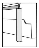
Use tall case protectors or posts, 24" or higher, to protect cases or fixtures with recessed bases.
