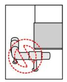
Do not install the case protectors or floor bumpers away from the case or fixture.
