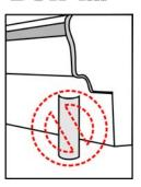
Do not use short case protectors or floor bumpers to protect cases or fixtures with recessed bases.
