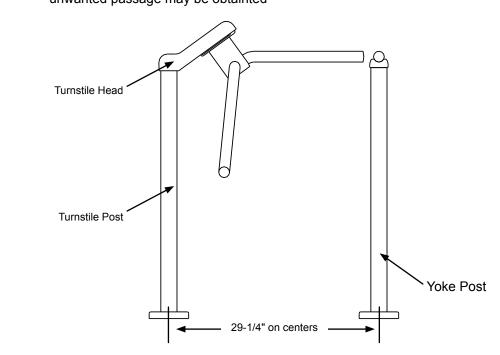
Anchor the posts per the vouge style or zenith style post installation instructions that are provided with this document. When using zenith style posts, completely tighten the outer four anchor bolts and ONLY SEAT the center anchor. Do not install the center anchor shaft at this time.
