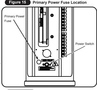
· Lower Column rotated to show power switch.
