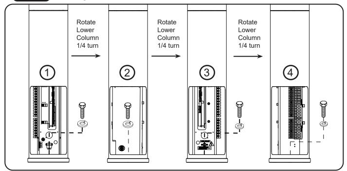
**NOTE** With the set screw loosened, the Lower Column can rotate freely.
