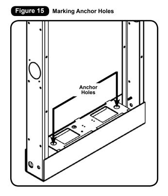
Using a 1" concrete drill bit, drill the anchor holes a minimum of 3" in depth at the center of each marked location.
