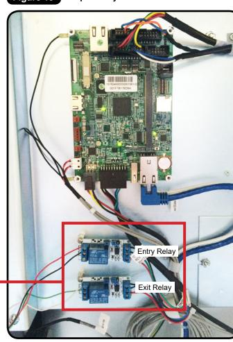
2. Using a precision flat-blade screwdriver, wire the relay's normally open (N.O) and common (COM) terminals to the GWCB-12 input terminals [Figure 19A].
