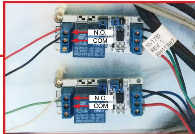
2. Using a precision flat-blade screwdriver, wire the relay's normally open (N.O) and common (COM) terminals to the GWCB-12 input terminals [Figure 19A].
