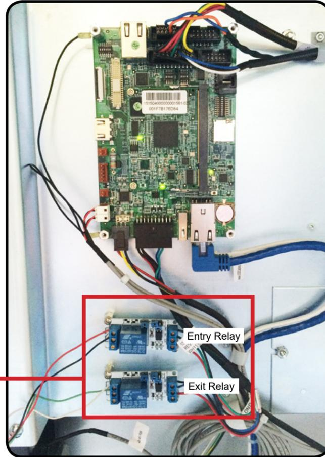
**Figure 19A** Output Relay Terminals
