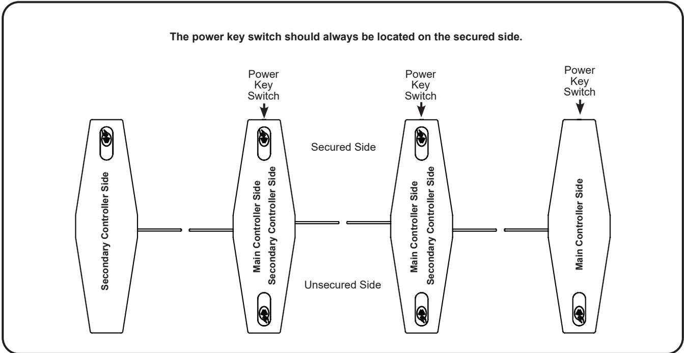
**Fig. 11** Incorrect Turnstile Layout
