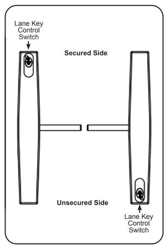
Turning the key to one of three positions overrides all existing settings, placing the turnstile in Controlled Passage mode, Free Passage mode or No Passage mode depending on the orientation of the key. Refer to the Passage Modes section on Page 15 for more information.
