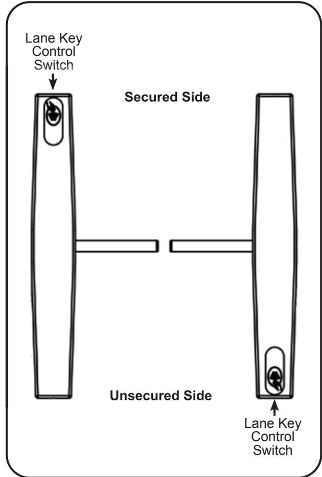
**Fig. 14** Lane Key Control Switch
