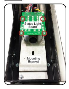
Fig. 17 Mounting Screws
