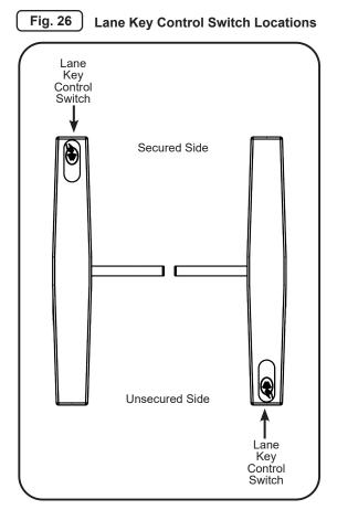
Turning the key to one of three positions overrides all existing settings, placing the turnstile in Controlled Passage mode, Free Passage mode or No Passage mode depending on the orientation of the key. Refer to the Passage Modes section on Page 24 for more information.
