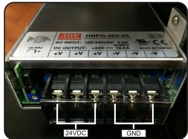
**Fig. C5 Turnstile Power Terminal Block**
