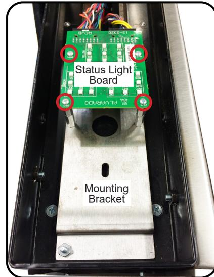
**Fig. 17** Mounting Screws
