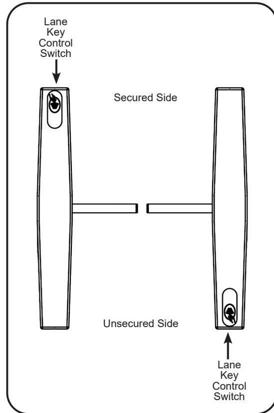
Turning the key to one of three positions overrides all existing settings, placing the turnstile in Controlled Passage mode, Free Passage mode or No Passage mode depending on the orientation of the key. Refer to the Passage Modes section on Page 24 for more information.
