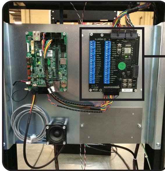
Figure 21A I/O Control Board (13-1328 Rev. F)
