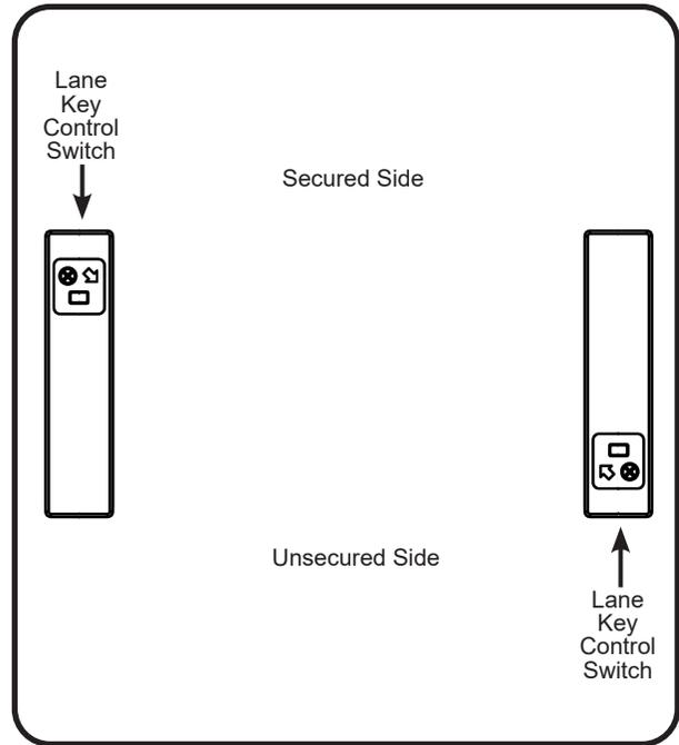
Turning the key to one of three positions overrides all existing settings, placing the turnstile in Controlled Passage mode, Free Passage mode or No Passage mode depending on the orientation of the key. Refer to the Passage Modes section on Page 24 for more information.
