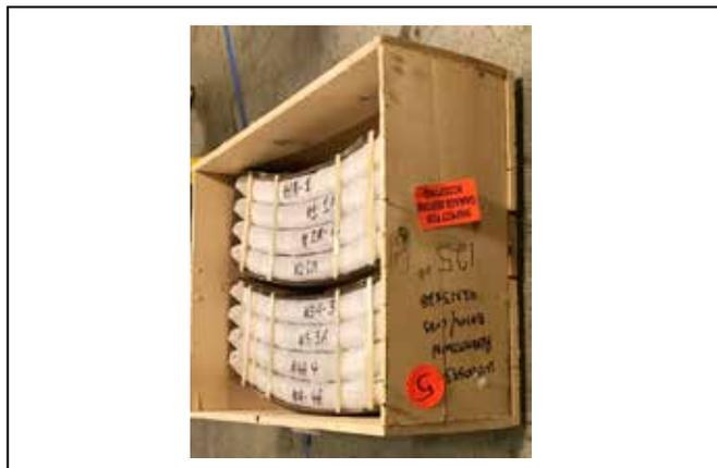
Fig. 19.1.3 Bottom rail numbering
