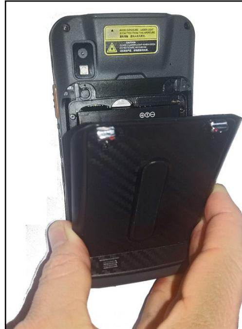
6. Secure the battery cover by rotating locking latches downward to the vertical, locked position.
