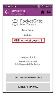
If a device scans a ticket in offline mode, that same ticket cannot be validated again by that device while the scan data is stored locally. After the device reestablishes its connection with the server, it uploads all offline scan data. The server determines whether the scans would have been valid or invalid if they were validated by an online device and stores those results in the database
