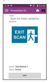
Enable or disable Exit Mode or the Entry/Exit Mode button on the Device Setup screen. See the <u>Device Setup Screen</u> section on page 18.
