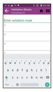
The *Validation Masks* screen allows operators to add, edit, or delete validation masks, if the device is not currently connected to the server. A validation mask is a pattern that ticket barcodes must match to be considered valid.
