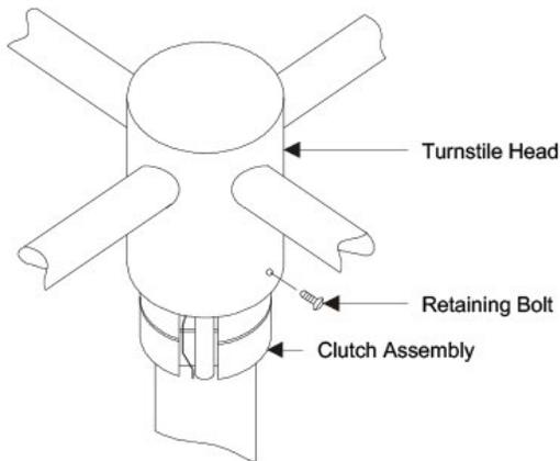
Installing the Turnstile Head.
