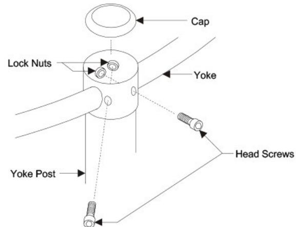
Installing the Yoke.
