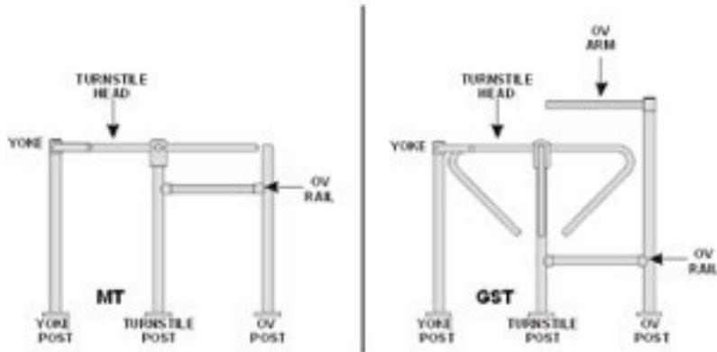
**NOTE** The product is ready for installation on level concrete assuming that no modifications are made to the product.
