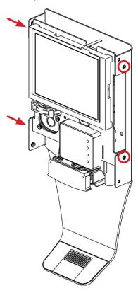
2. Secure the backplate to the wall using appropriate mounting hardware. Pull the Ethernet cable and door strike wires through the open area for conduit wiring on the back plate while you do so.
