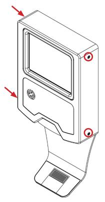
4. When the case is attached, access the power button through the opening on the lower-right side of the unit.
