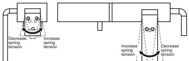
**Appendix E - Fail-lock / Fail-safe Spring and Solenoid Configurations (Cont)**
