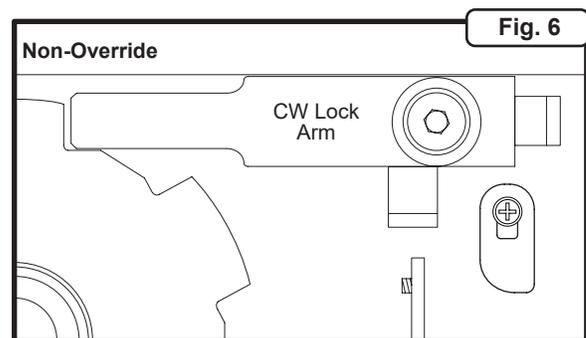
2. Rotate key back to non-override position, verify lock arm engages cam shaft lobe and key is removable (Figure 6).
