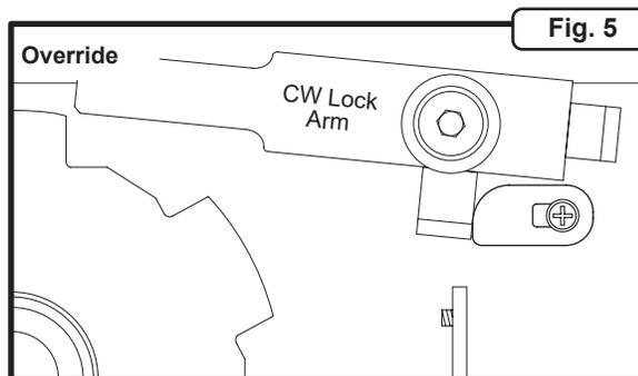
1. Rotate key to override position, verify lock arm clears cam shaft lobe and key is removable (Figure 5).
