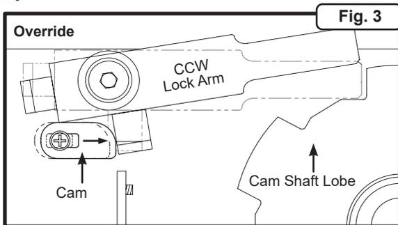
1. Hold CCW lock arm open and rotate the key to the override position (Figure 3).
