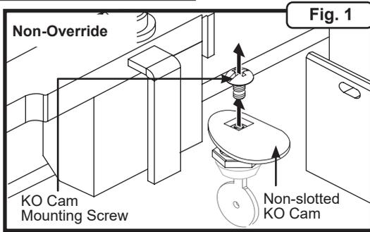
1. Rotate the key lock to the non-override position; then remove non-slotted key override (KO) cam (Figure 1).
