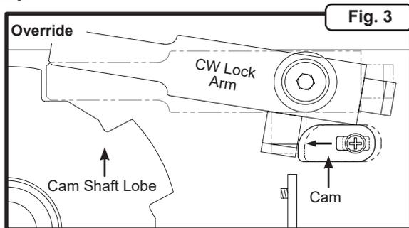
1. Hold CW lock arm open and rotate the key to the override position (Figure 3).
