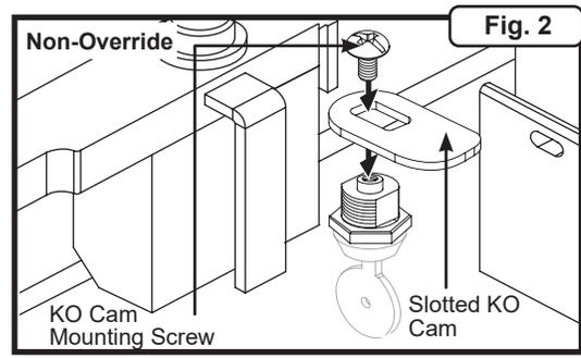
2. Install slotted KO cam. Do not fully tighten at this time (Figure 2).
