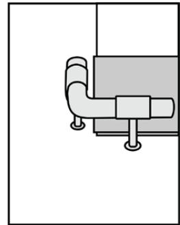
Install the case protectors or floor bumpers as close as possible to the fixture being protected.
