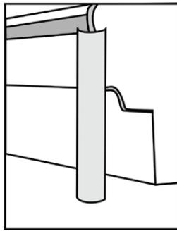
Use tall case protectors or posts, 24" or higher, to protect cases or fixtures with recessed bases.
