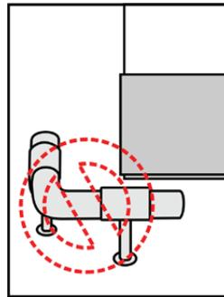
Do not install the case protectors or floor bumpers away from the case or fixture.
