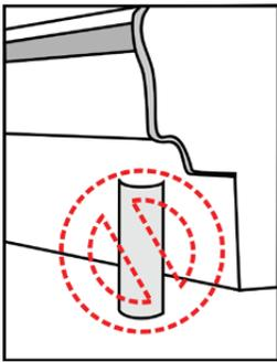
Do not use short case protectors or floor bumpers to protect cases or fixtures with recessed bases.
