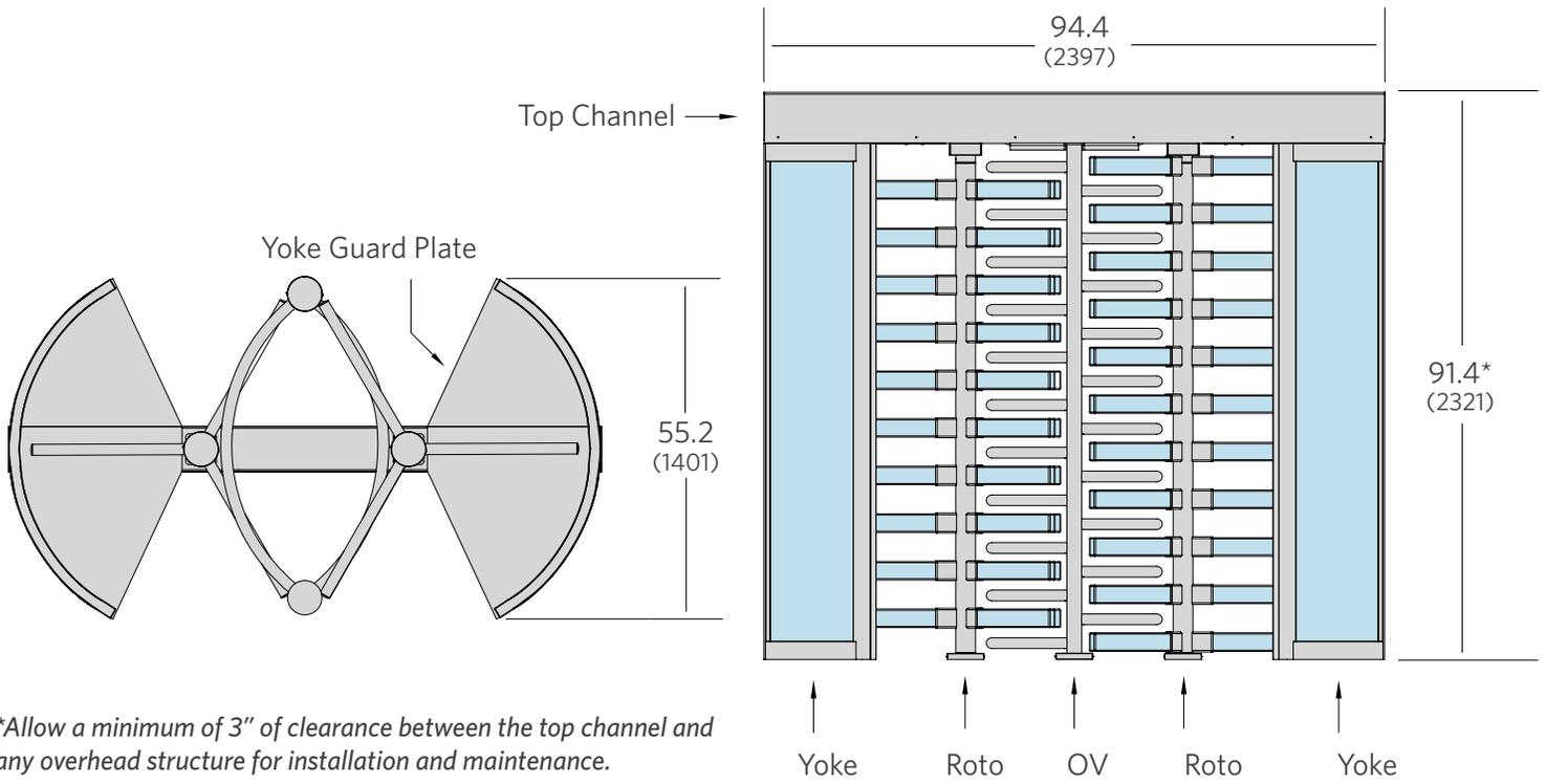
*\*Allow a minimum of 3" of clearance between the top channel and any overhead structure for installation and maintenance.*
