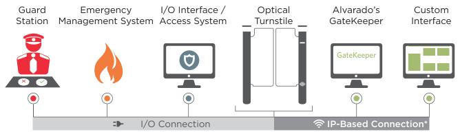
\*IP-based gate control operates with Alvarado's GateKeeper or with any interface.
